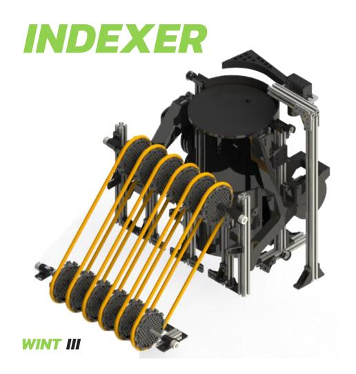
Uses same HD motor as intake geared down 20:1 to move rings inside the robot.
