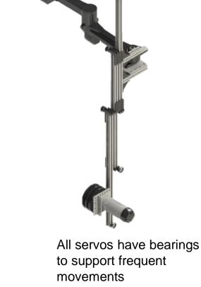
Elevator that can rise up to 70cm driven by a HD motor geared 40:1 to get a full extensión in les tan 0.5 seconds.
